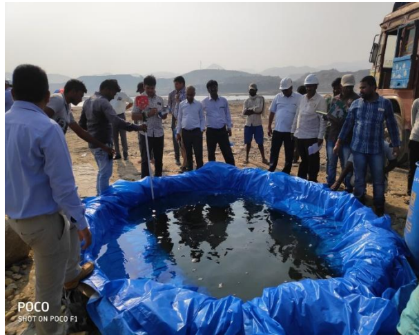
In-situ density of rockfill material using water replacement method
