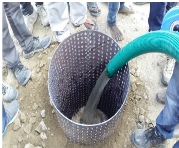
Field Permeability test
